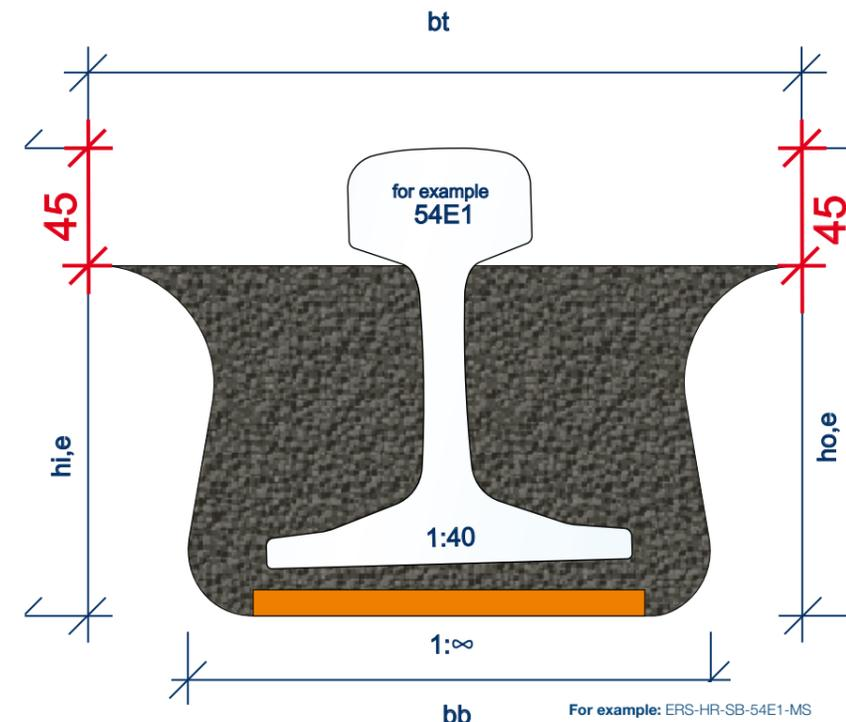
Group SB versions of ERS rail fastening systems are designed for applications in combination with steel module bridges (MB-S), or with modular steel deck plates.
