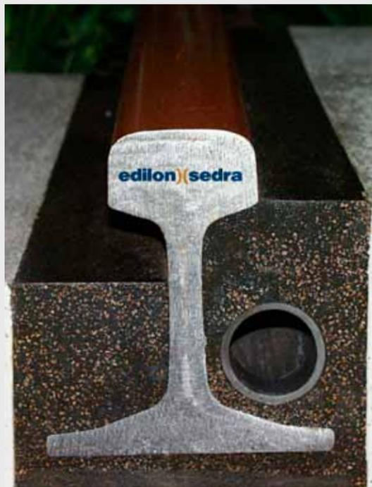
The ERS rail fastening system is characterized by continuous support of the rails, as well as by the elimination of any and all forms of small hardware components. This also means avoidance of the support-point frequencies of traditional, discrete rail fastening systems – and it enables transfer of live traffic loads more uniformly and with reduced load peaks into the supporting track substructure.
